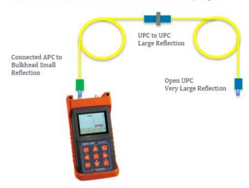
The 930XC with an APC bulkhead and an APC to UPC 1m jumper
