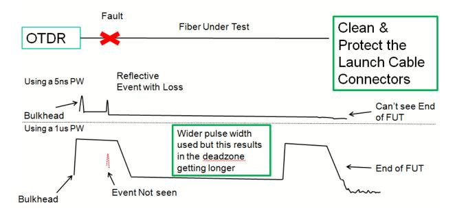
Here you can see that with a 5ns pulse width the fault can be easily measured but the end of the fiber can't be seen. If a wider pulse width is used (1us) the fault can no longer be measured. This is because the event deadzone has become too long and the bulkhead and fault are now represented as one pulse.
