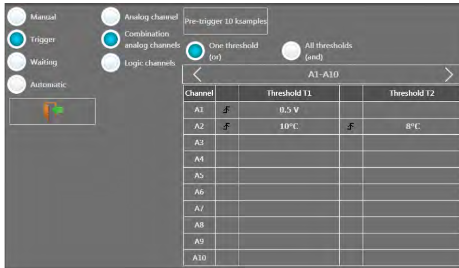
Figure 8.5 Multiple Threshold Trigger Screen
