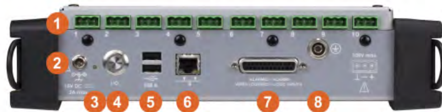
Figure 1.2 DAS240-BAT Electrical Connections
