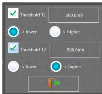
Figure 9.5 Alarm Analog Thresholds
