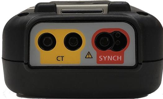
The current clamp plugs into the CT inputs.
