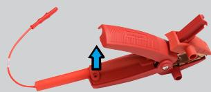
Then pull back to remove the guard and expose the fuse
