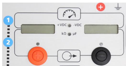
Once the transmitter had completed booting the lower left voltage display will be flashing.
