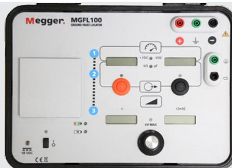
Connect the green terminal to the IT Filter box input.
