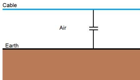
Add this to the capacitance already on the system due to equipment on the system and it is clear that the capacitance on these systems can get to substantial levels.
