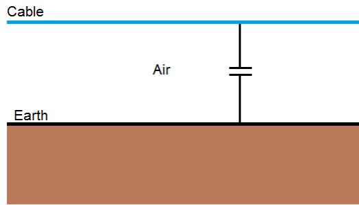
In addition, capacitance is already on the system due to equipment on the system. It is clear, therefore, that the capacitance on these systems can exist at substantial levels.
