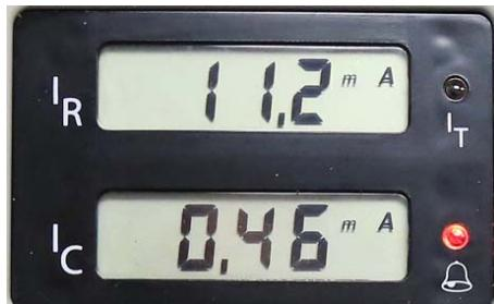
If the reactive current is higher than the fault current, then this circuit is only drawing current due to capacitance and the fault is on another circuit.
