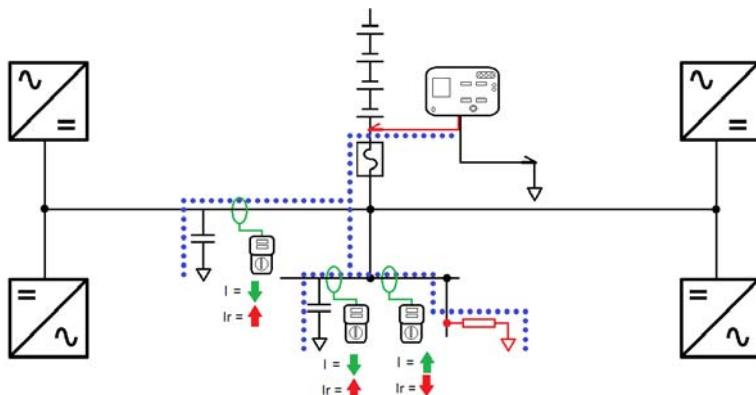
This allows one to see which circuit(s) is drawing current due to a fault(s) and which is drawing current due to high levels of capacitance.
