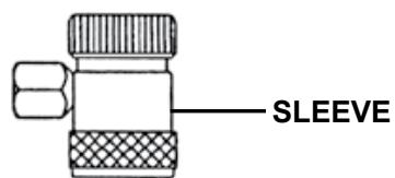
To attach to the system, make sure that the coupler is in its unlocked position. Press the coupler against the service port until it snaps (locked position).
