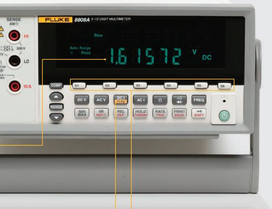
i-Lkg function adds two additional hi-impedance ranges for sensitive low current measurements
