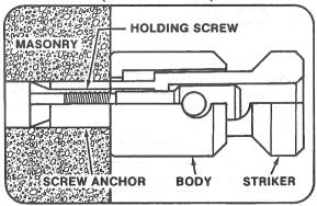
Screw Anchor Expanders--Hardened alloy steel.
