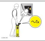
7. At a distance of 5 m (16 ft) to the connection point, circle around the connection point.
