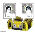
3. Place the transmitter over the utility with the arrows running in line with the suspected direction of the utility.
