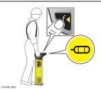
7. Walk in line with the suspected direction of travel observing the display. The signal strength indicator rises and falls as you pass over the ghost signal at the back of the sonde, the peak signal directly over the sonde and the ghost signal at the front. The Numeric Peak Indicator displays its highest value when detecting the peak signal.
