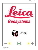
This screen allows you to adjust the time zone settings to suit your geographic region. The default time is Universal Time Coordinate (UTC). Time zone offsets are shown in Appendix A Time Zone Offsets. Set up the hours and minutes.
