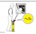
8. Sweep the area until a signal is detected. Pinpoint and trace the utility.
