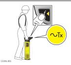
5. Using the Sweep Search process, search the work area until either a signal is detected or you are satisfied that the area has been adequately tested.
