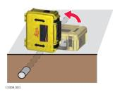
3. If the transmitter and the locater are on the same utility, the Numeric Peak Indicator on the locator significantly decreases.
