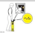
7. At a distance of 5 m (16 ft) to the connection point, circle around the connection point.
