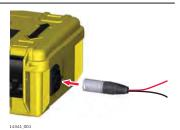
3. Connect the red cable to the positive (+) terminal on the trace rod. Connect the black cable to the negative (-) terminal.
