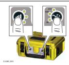
6. Set the locator to Signal Transmitter mode and select the required frequency.
