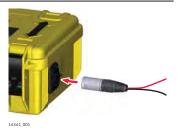
2. Ensuring that no utilities are below, push the Earth Pin into the ground and connect the black cable to the Earth Pin.
