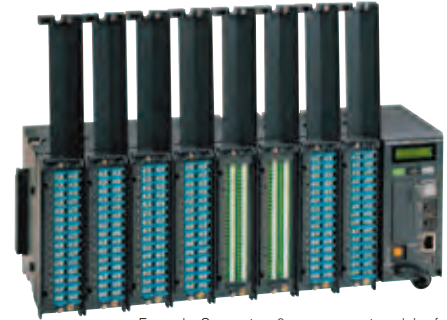
Example: Connect up 8 measurement modules for a 120-channel system
