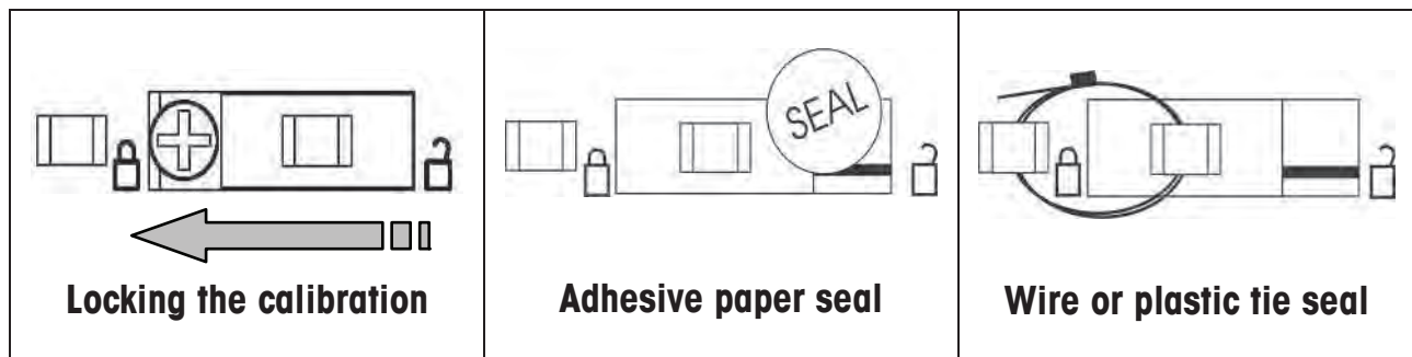
Figure 4-1. Locking and Sealing the Calibration Lock Switch.
