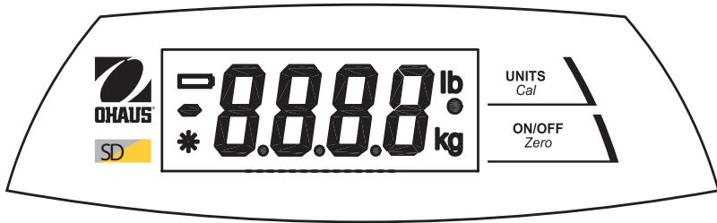
Figure 5. Indicator Panel Controls.
