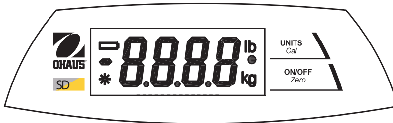
Figure 5. Indicator Panel Controls.
