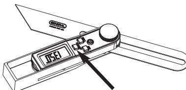
Press the HOLD/FLIP button for 3 seconds to invert the display
