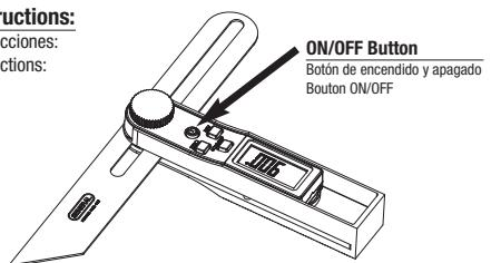
To clear the display to zero, make sure the blade is completely closed into the handle and press the zero button
