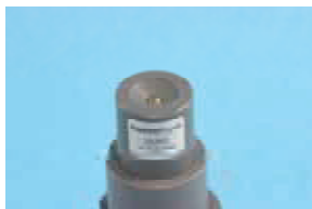
Zero calibration standard with target ball put on it
