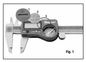
First, unscrew and remove the battery cover (1) by turning it to the left  $\frac{1}{2}$  turn. Remove the old battery. Next, position the rubber "0" ring (3) correctly in the bottom of the battery compartment before inserting the new battery (2) negative side (-) down. Then, re-install the battery cover (1) and lock it into position by giving it a  $\frac{1}{2}$  turn to the right.
