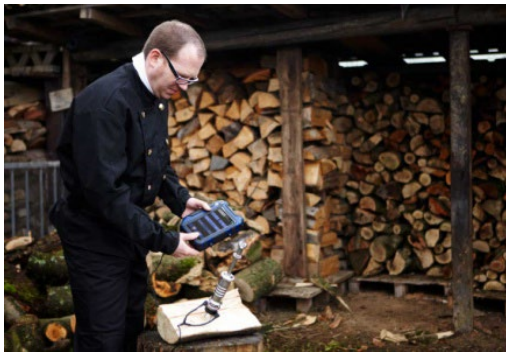
Fig. 40: Wood moisture measurement with Probe Wöhler HBF 420.
