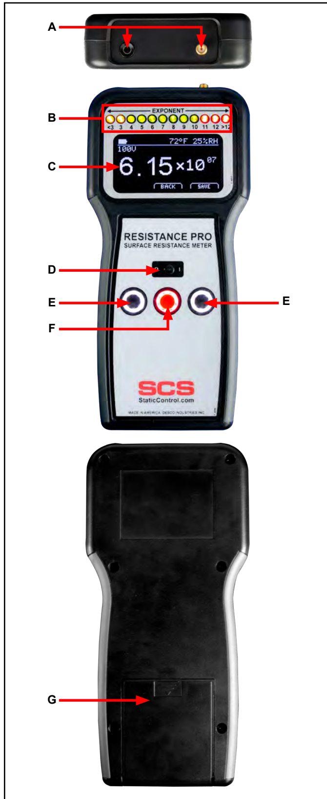
Figure 4. Resistance Pro Meter features and components
