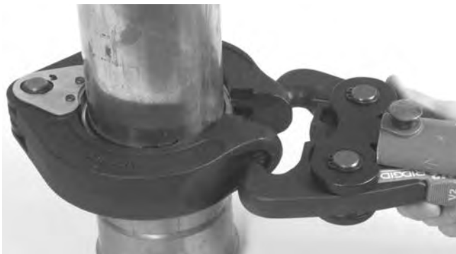
Figure 14A – Placing V2 Actuator Tips Into XL-C Ring Pockets
