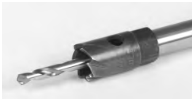
Figure 5 – Installation of pilot drill
