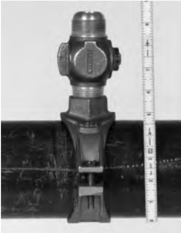
Figure 10 – Measuring maximum stroke
