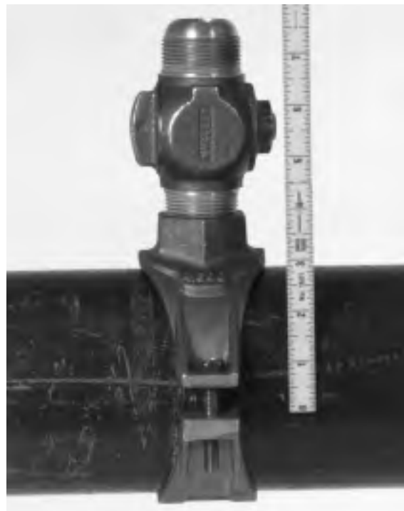
Figure 9 – Measuring valve standoff distance
