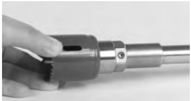
Figure 3a – Installation of large hole saw adapter
