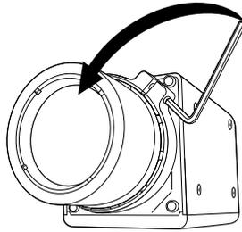
2. Focus the camera by rotating the lens.
