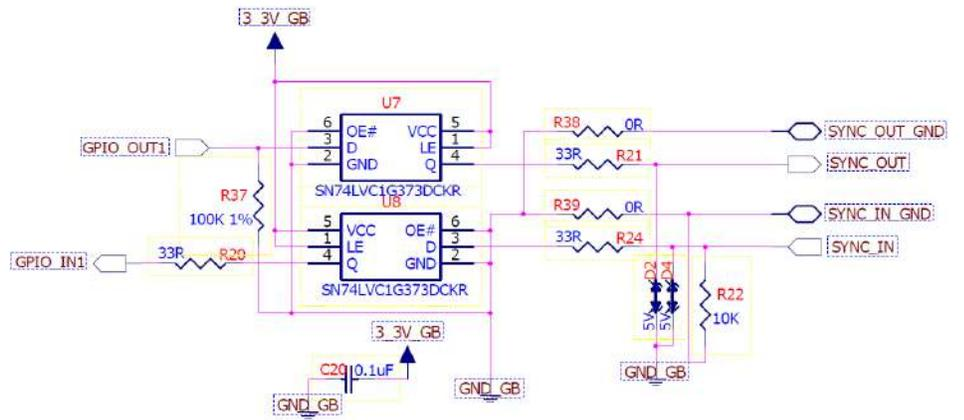
Figure 16.3 Schematics of SYNC input and output.
