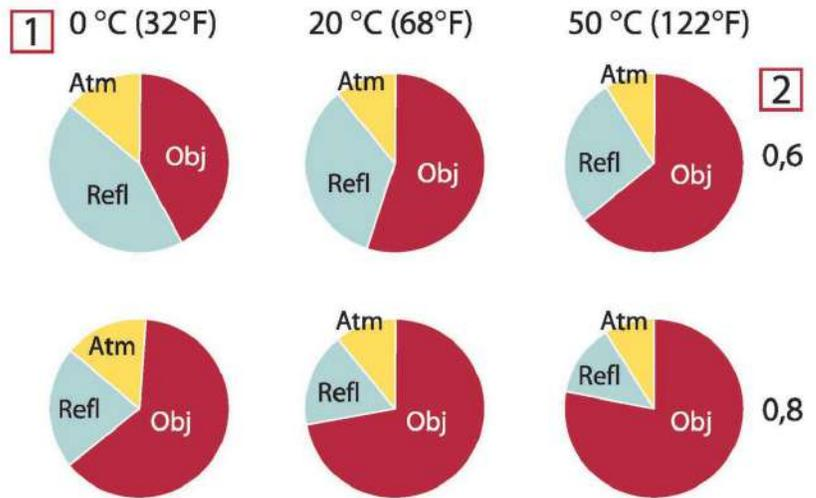
**Figure 23.3** Relative magnitudes of radiation sources under varying measurement conditions (LW camera). 1: Object temperature; 2: Emittance; Obj: Object radiation; Refl: Reflected radiation; Atm: atmosphere radiation. Fixed parameters:  $\tau = 0.88$ ;  $T_{refl} = 20^{\circ}\text{C}$  (+68°F);  $T_{atm} = 20^{\circ}\text{C}$  (+68°F).
