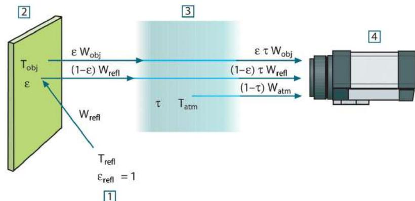
**Figure 23.1** A schematic representation of the general thermographic measurement situation. 1: Surroundings; 2: Object; 3: Atmosphere; 4: Camera
