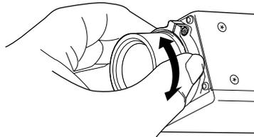
3. Lock the clamp by tightening the Allen screw.
