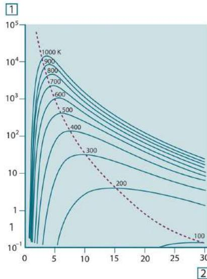
**Figure 22.6** Planckian curves plotted on semi-log scales from 100 K to 1000 K. The dotted line represents the locus of maximum radiant emittance at each temperature as described by Wien's displacement law. 1: Spectral radiant emittance ( $\text{W}/\text{cm}^2\ (\mu\text{m})$ ); 2: Wavelength ( $\mu\text{m}$ ).
