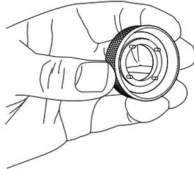
2. Align the four pegs with the corresponding slots on the front of the lens, and push the focus adjustment tool into position.
