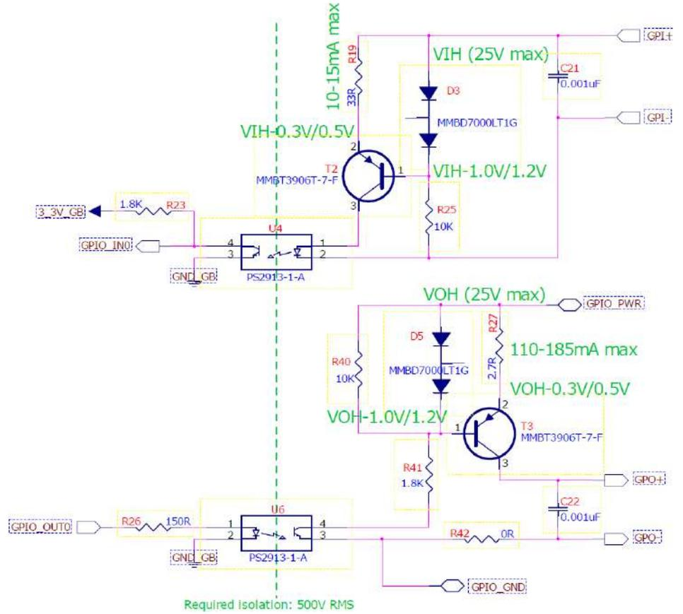
Figure 16.4 Schematics of GP input and output.
