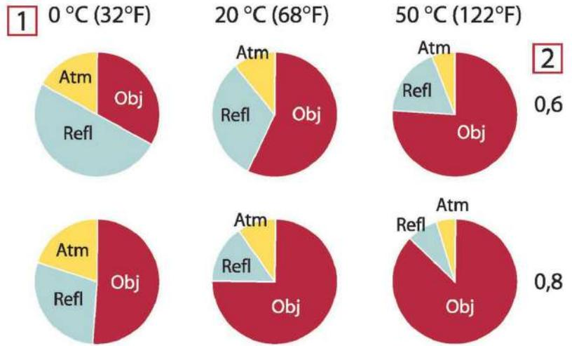
**Figure 23.2** Relative magnitudes of radiation sources under varying measurement conditions (SW camera). 1: Object temperature; 2: Emittance; Obj: Object radiation; Refl: Reflected radiation; Atm: atmosphere radiation. Fixed parameters:  $\tau = 0.88$ ;  $T_{refl} = 20^{\circ}\text{C}$  (+68°F);  $T_{atm} = 20^{\circ}\text{C}$  (+68°F).
