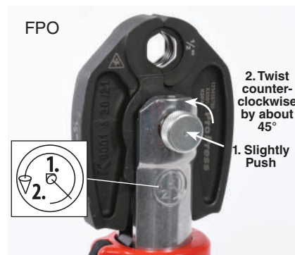
Figure 7 – Opening The Attachment Mounting Pin
