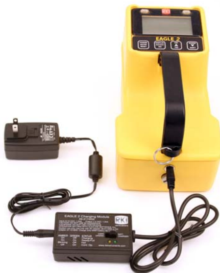
Figure 17: Connecting the EAGLE 2 to the Charger
