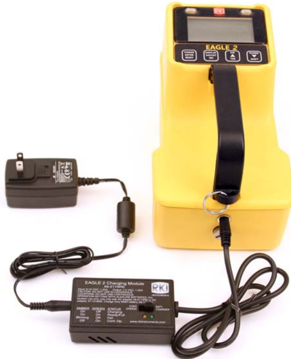
Figure 20: Connecting the EAGLE 2 to the Charger
