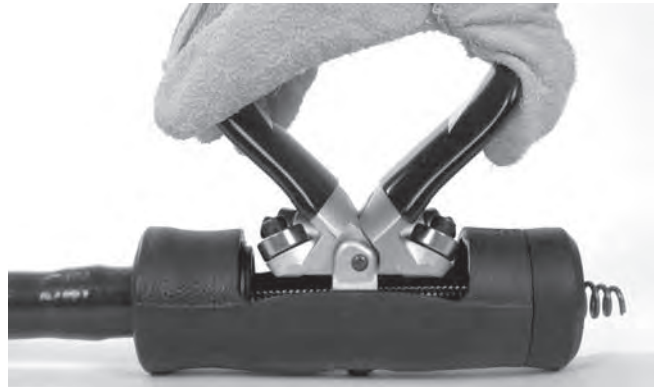
Figure 5 – Feeding cable through AUTOFEED
