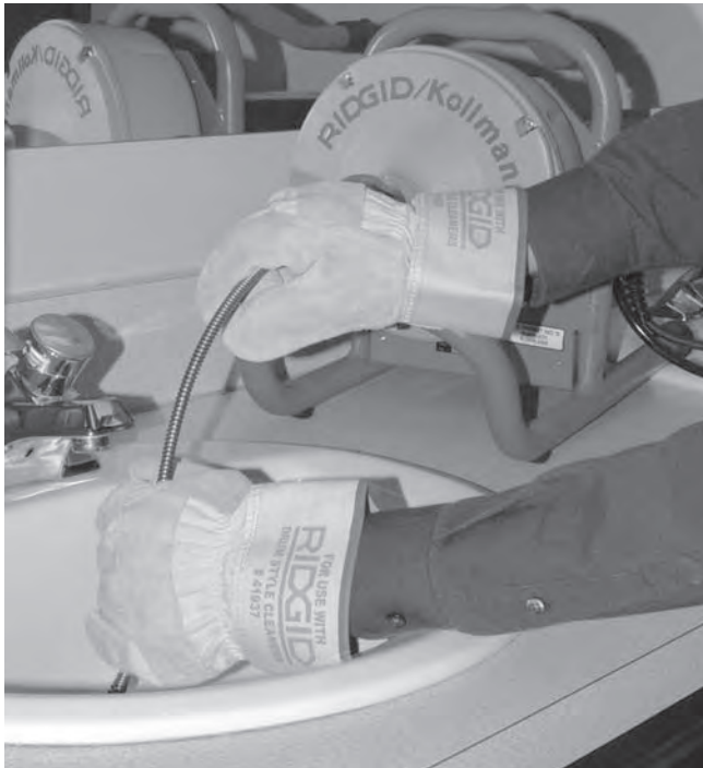
Figure 11 – Manually Feeding Cable
