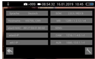
Fig. 54: Info menu with SOM (Firmware of the camera) and CAM (Version of the camera head)
