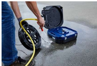
Fig. 77: Cleaning the viper and the rod
