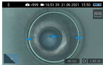
Fig. 45: Distance between 2 measuring points
