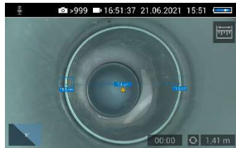
Fig. 46: Warning triangle under distance indicator
