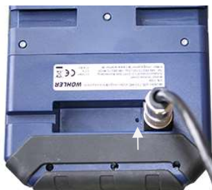
Fig. 69: Reset hole indicated by an arrow
