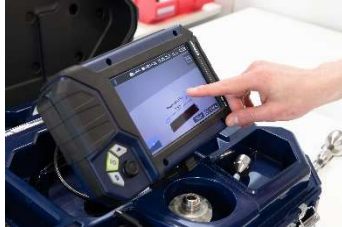
Fig. 47: The measuring points can be moved by dragging them
