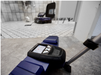
Precise location of the camera head with the Wohler L 200 Locator.
