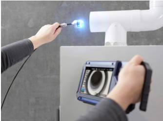
Inspection of flue gas lines from 2"; easily negotiates tight bends of 87°.
