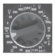
**NOTE:** When in a Resistance setting and the test leads are open (not connected across a resistor), or when a failed resistor is under test, the display will indicate O.L. This is normal.
