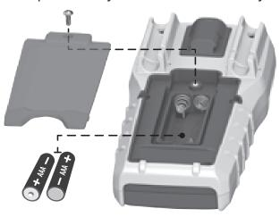
To avoid risk of electric shock, disconnect leads from any voltage source before removing battery door.
