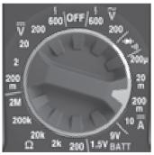
3. To measure current: Remove power from circuit, open circuit at measurement point, connect meter in-series in the circuit using the test leads, and apply power to circuit. The meter will autorange to display the measurement in the most appropriate range.
