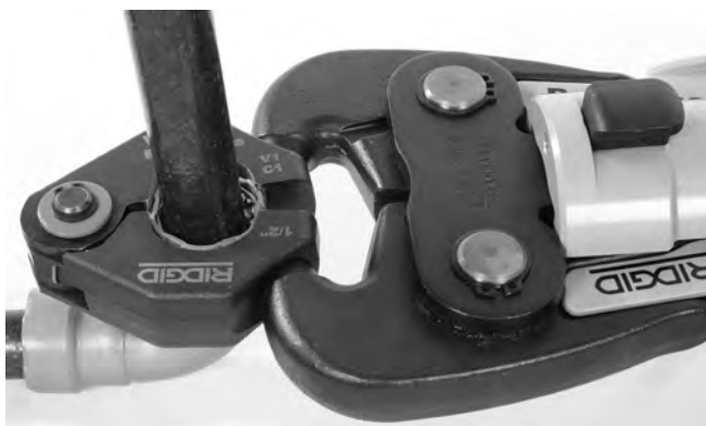
Figure 12 – Attaching Actuator to Press Ring
