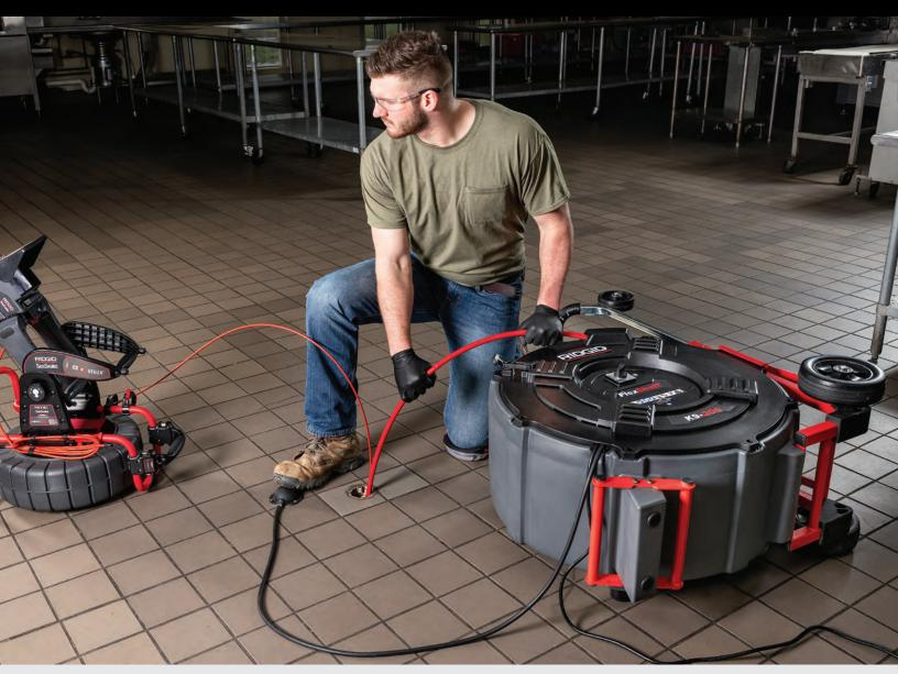
Purpose-built for the professional, the RIDGID® FlexShaft K9-306 quickly clears grease buildup, roots and heavy scale using 125' of 3/8" cable for 3" - 6" pipes with one step of the foot switch. It features a professional 1.5 HP internal universal motor for maximum power and longevity, a fully enclosed drum to minimize set-up and clean up time, and a telescoping handle with multiple wheels and grab points to make loading, unloading, transporting, and storage easy.
