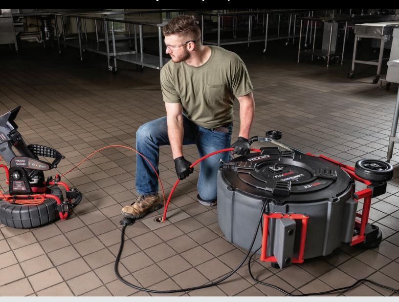
Purpose-built for the professional, the NEW RIDGID® FlexShaft K9-306 quickly clears grease buildup, roots and heavy scale using 125' of 3/8" cable for 3" - 6" pipes with one step of the foot switch. It features a professional 1.5 HP internal universal motor for maximum power and longevity, a fully enclosed drum to minimize set-up and clean up time, and a telescoping handle with multiple wheels and grab points to make loading, unloading, transporting, and storage easy.
