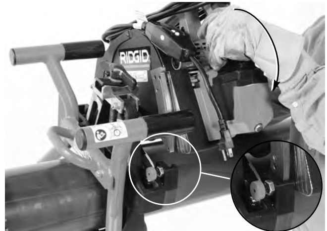
Figure 12 – Engaging Plunge Plate Into Guide
