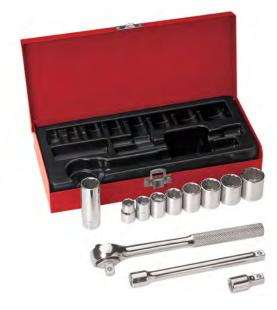
This 12-piece Wrench Set includes four 6-point and four 12-point sockets. 6-point socket sizes include 3/8-lnch, 7/16-lnch, 1/2-lnch and 9/16-lnch. The four 12-point sockets span 5/8-lnch, 11/16-lnch, 3/4-lnch and 13/16-lnch sizes. Also, includes a 5/8-lnch spark plug socket, two extensions and a ratchet. Keep all of pieces together in a compact hinged metal box.
