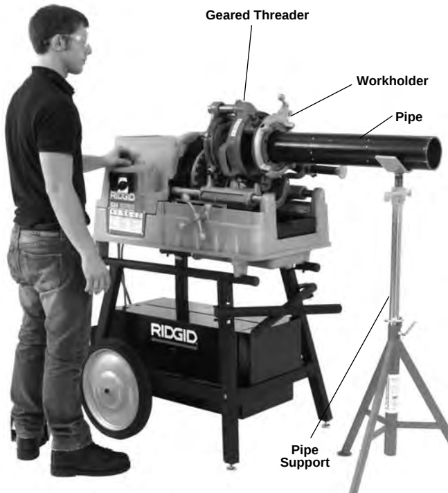
Figure 21 – Operating Position (Close-Coupled Method)
