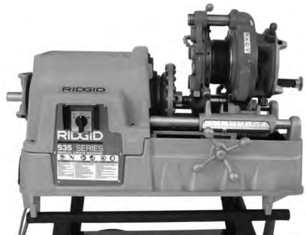
Figure 17 – Geared Threader Close-Coupled To 535
