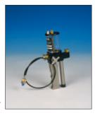
System C is an easy-to-use single hand-operated calibration system. No need for a flat surface (table) to operate the system. The system includes release valve and vernier valve for fine adjustment to enable safe and simple operation of the pump.
