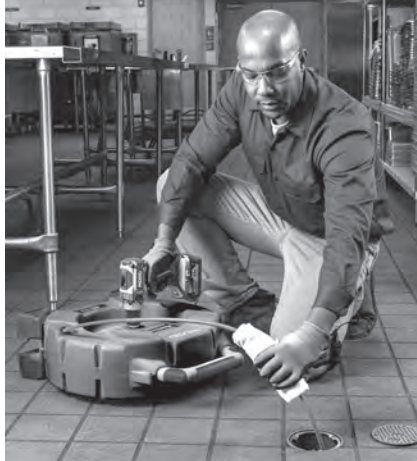
Figure 13 – Applying Lubricant to the Cable Sheath
