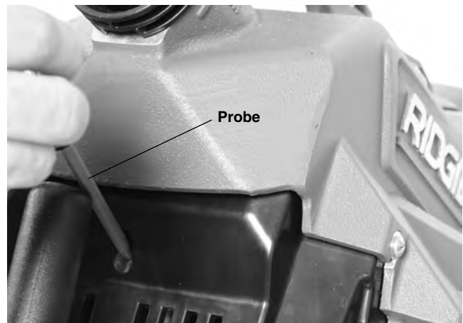
Figure 22 – Motor Reset Button
