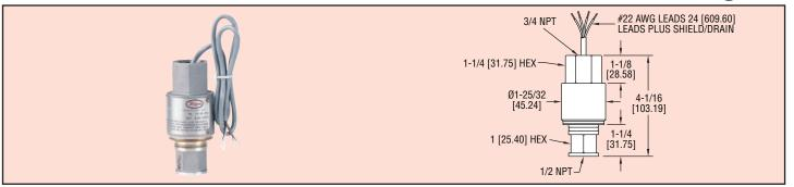
The Series 636 Pressure Transmitter is a low cost, fixed range, stainless steel transmitter with  $\pm 0.30\%$  accuracy. It is designed to continuously measure pressure for years in even the toughest environmental and media conditions. Select from 4 ranges to 0 to 300 psig (0 to 20 bar) with choice of 4 to 20 mA output (model 636) or 1 to 5 VDC output (model 636LP). Transmitters are explosion-proof, (FM approved) and meet NACE standards for offshore applications.
