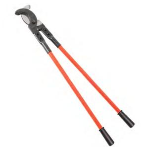
Klein Tools' Communcation Cable Cutter is a lightweight, yet efficient shear-type cable cutter. It is designed to cut up to 900-pair soft copper and aluminum cable, and also lead or rubber-covered communcations cable. Forged steel jaws make a clean, even cut for ease in fitting lugs and terminals.
