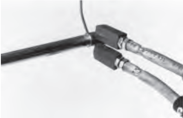
Figure 7 – Soldering with Carbon Tips Contacting Fitting
