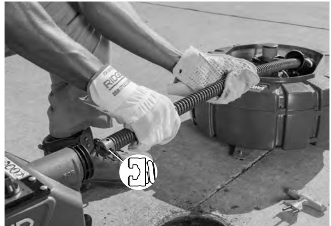
Figure 7 – Inserting Cable Into Front Of Machine
