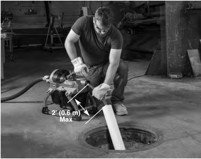
Figure 5 – Example of Extending Drain to within 2' of Machine Cable Outlet
