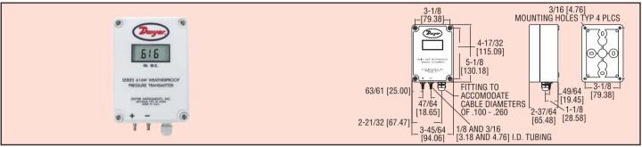
The Series 616WL Differential Pressure Transmitter senses very low pressures of air and non-combustible, compatible gases and sends a standard 4-20 mA output signal. All models, including those featuring the 3 digit LCD digital read-out, are factory calibrated to specific ranges as listed in the chart below.
