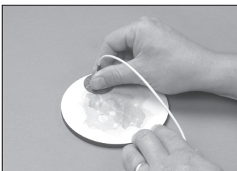
11.19 Polish the connector for four to eight figure eights only.
