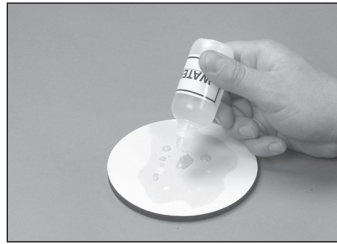
11.14 Final Polish: Clean the lapping film with a lint free cloth and distilled water. Add several drops of distilled water onto the lapping film.
