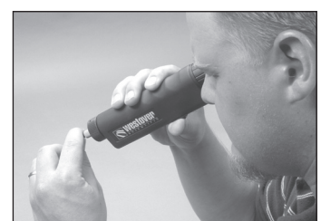
11.21 Inspect the connector endface with the fiber through coaxial and oblique views by changing the view with the thumbswitch on the body of the 3M View Scope.
