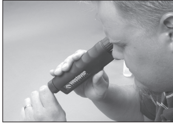
10.11 Inspect the connector endface with the fiber through coaxial and oblique views by changing the view with the thumbswitch on the body of the 3M View Scope.
