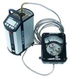
The tall CTC models with an immersion depth of 190 mm / 7.5 in are ideal for calibration of liquid filled sensors. The specially designed non-linear heating elements in the CTC-650 B and the increased block mass provide a very homogeneous temperature throughout the block. It is essential for the quality of the calibration/test that the full length of the sensing part of the sensor is exposed to the same temperature. Calibrate analog reading devices or switches with very high repeatability.
