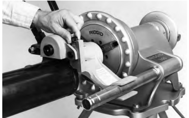
Figure 10 – Loosen Depth Adjustment Screw
