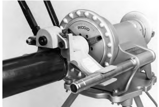
Figure 9 – Feed Handle in UP Position
