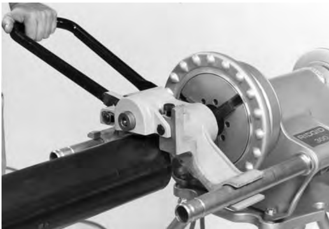
Figure 12 – Forming the Roll Groove
