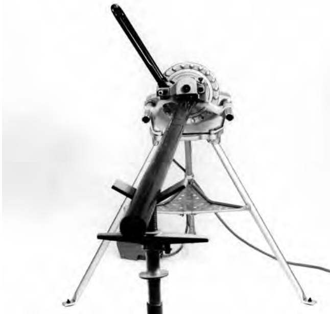
Figure 8A – Operating Machine in REVERSE (REV) Position
