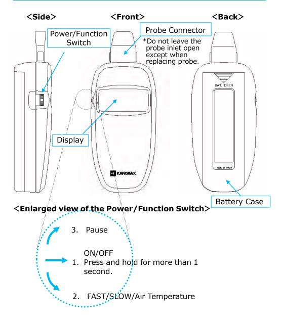
Power/Function Switch is a multifunction switch that can be slid up and down, and pressed.
