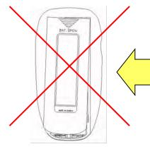
To put the battery cover back, do not first engage the detent at the top end.
