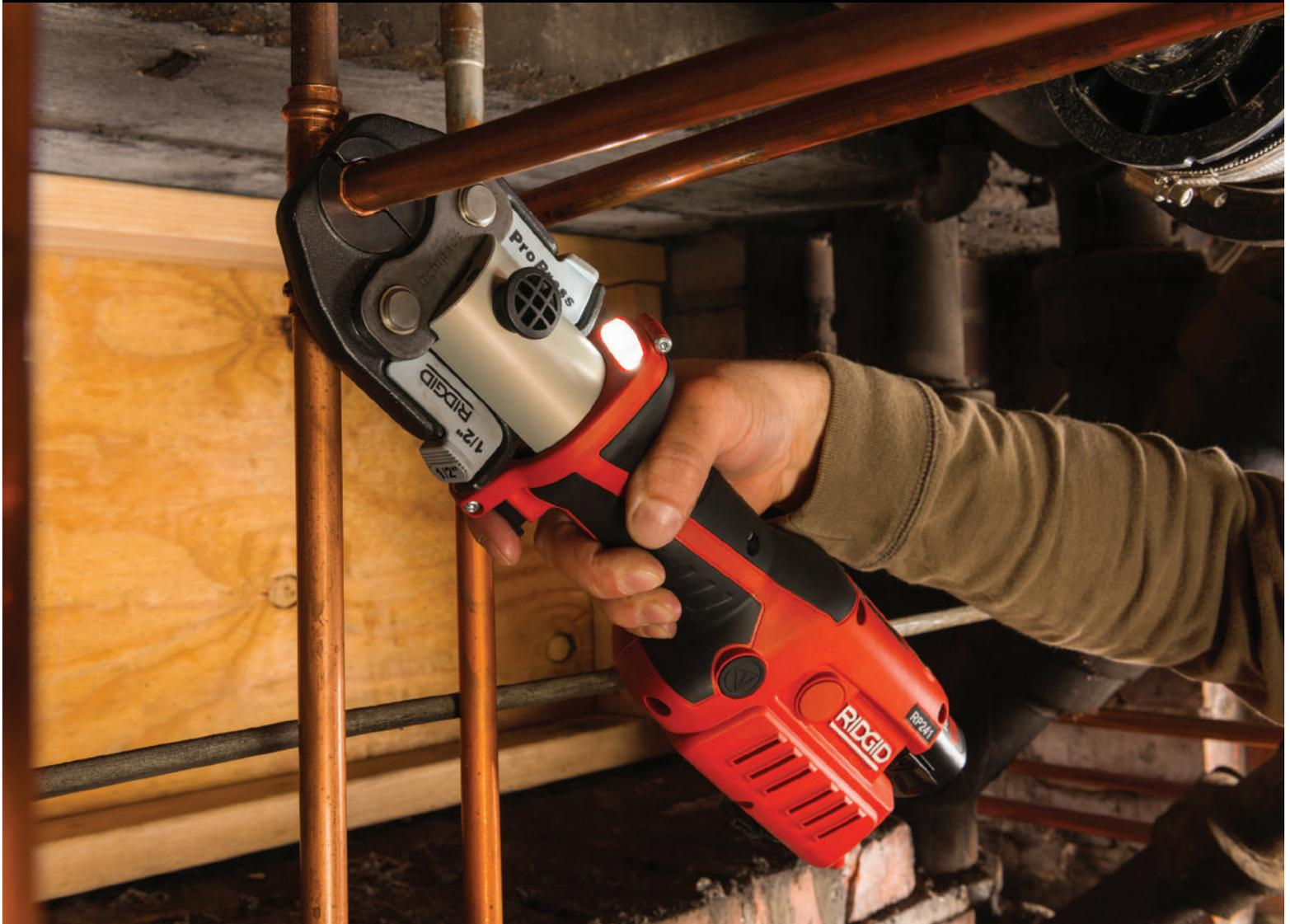
**The RP 240 & RP 241 are the latest tools in the RIDGID® Compact Press Tool family. Up to 25% smaller and 10% lighter than their predecessors (RP 210 & RP 200), these lightweight, low profile designs, are ergonomically designed to help you easily work overhead and in tight spaces.**
