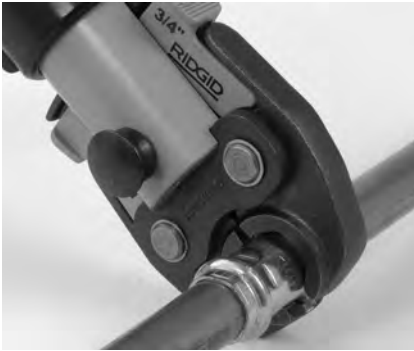
Figure 7 – Placing Scissor-Style Jaws Around Fitting
