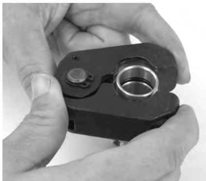
Figure 9 – Installing Press Ring onto Fitting
