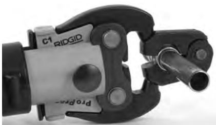
Figure 10 – Attaching Actuator to Press Ring
