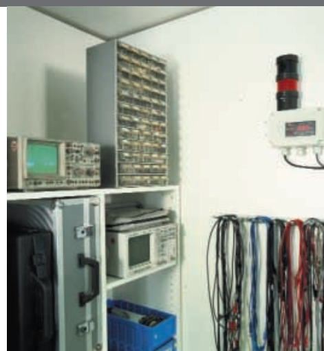
The two relay outputs of the testo 54 enable decentralized alarms when limit values are exceeded, e.g. with the help of the alarm column
