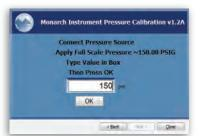
The software detects the full scale value and asks for a pressure source to be applied at that approximate value.
