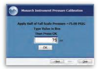
Some loggers support two point calibrations, and some support three points. The software automatically detects which is appropriate and prompts the next appropriate step. In a three point calibration, an adjustment is allowed for approximately mid-range.
