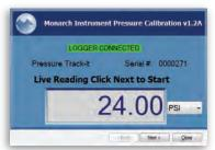
**Track-It™ Pressure Calibration Software** is a software Wizard, it automatically prompts you through the step-by-step procedure to perform vour calibration.
