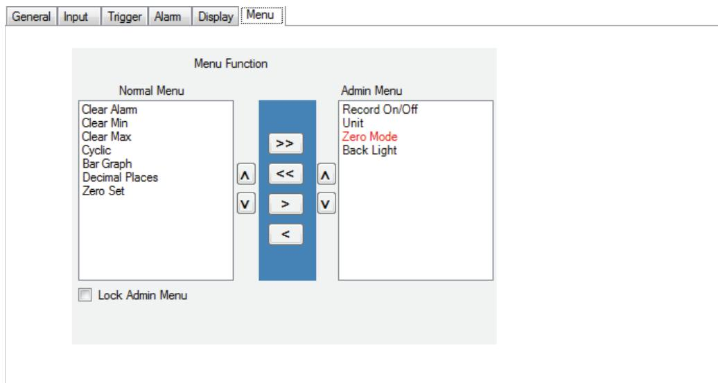
If the "Lock Admin Menu" box is checked the user will not be able to access the Admin Menu features at the Logger, and the Zero Set menu option (display offset) will not be available in the Normal Menu.
